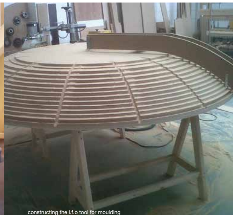
constructing the i.f.o tool for moulding
